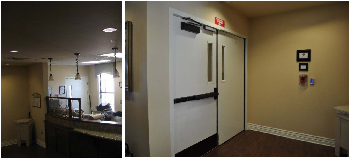
Images 8 & 9. Service entries into the unit. The door into the kitchen is a single door for food delivery. The double doors on the other side of the kitchen provide entry for large bins and equipment.
