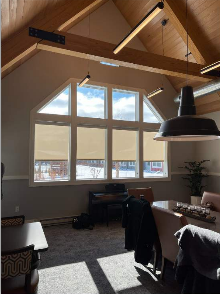
The conference room windows let in abundant light, but the non-shaded upper windows sometimes cause excess glare.
